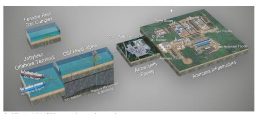
Figure 2. Pilot's MWCEP overview schematic
